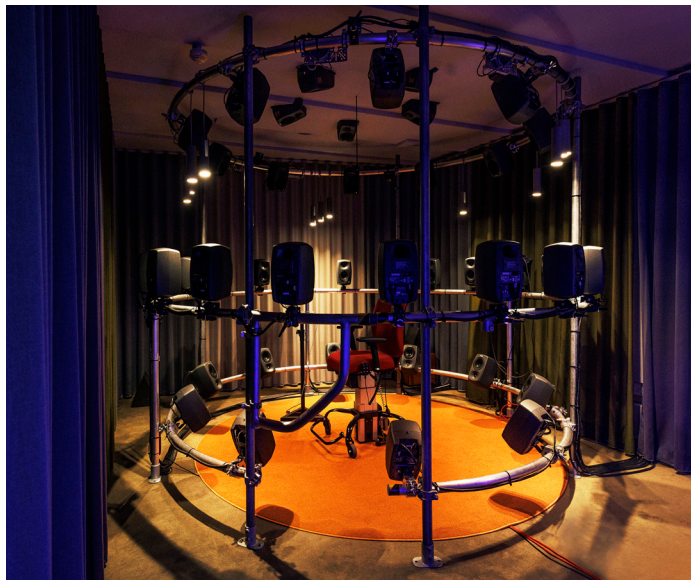
Figure 1: The speech-in-noise test was performed in the Spatial Audio Laboratory, consisting of 45 loudspeakers placed on 4 rings.
